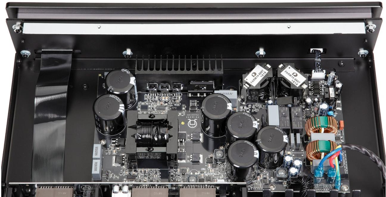
The internal structure is clearly arranged and equipped with a lot of SMD components. The coils can be found in all Class D amplifiers for filtering purposes.
